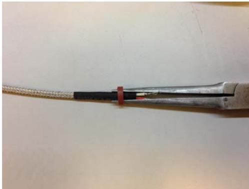
4. Put the clear ring and connect the wire to the connector
